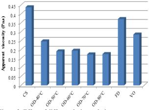
Figure 2. Effect of different drying techniques on apparent viscosity of Basil seed gum (shear rate=54s<sup>-1</sup>); control sample (CS), oven drying (OD), freeze drying (FD), and vacuum oven drying (VO).
